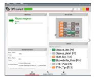
Run Status Screen (RSS) shows progress of run, current activity and time to completion
